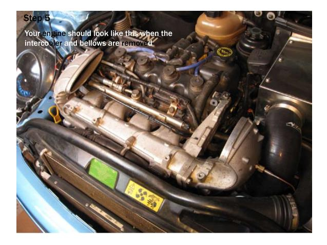
**Re-Install OEM bellows or install silicone** intercooler boots. - Slide DoS A2A-IC (IC). into outlet side intercooler boot. - Work the IC into supercharger (SC) side intercooler boot by tilting SC side boot slightly upward and then pushing both parts downward onto the SC side IC horn. If this does not work, a nonmarring nylon pry tool may help to ease the IC into the boot.
